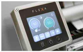
Automatic vertical alignment control panel
