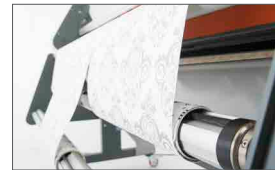
Front rewinding system: it rewinds the cut media up to three smaller rolls (optional for Miura Plus 160)
