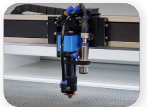
Hovering optic head with ultrasonic autofocus
